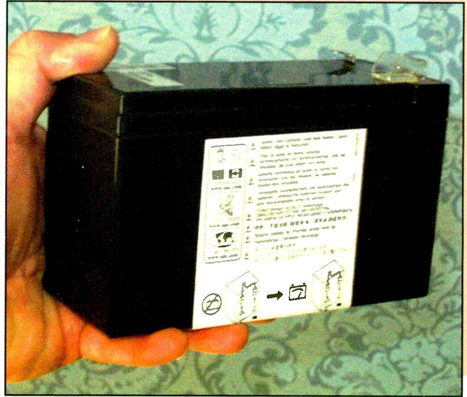
A small 7.5-amp-hour sealed battery taken from a back-up UPS unit.
