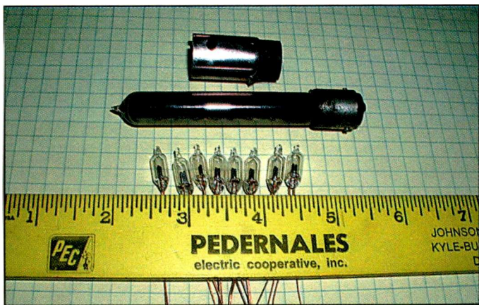
Photo A. The defunct Atwater Kent Tonebeam is shown with its socket and the eight neon lamps that were used to replace it.
