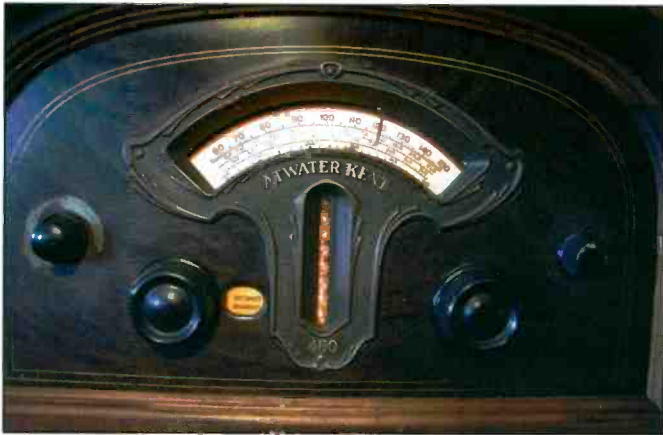
Photo F. The Atwater Kent is tuned to WOAI, a local 50-kW broadcast station, bringing the display to full height.
