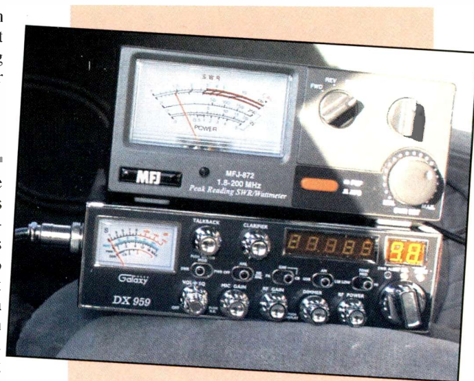
The Galaxy DX 959 ready to be installed. Note that in bright sunlight the radio's displays get washed out and are difficult to read. Checking the SWR on Channel 19 with the MFJ meter shows a 1.5:1 reading using the K40 Trucker antenna.
