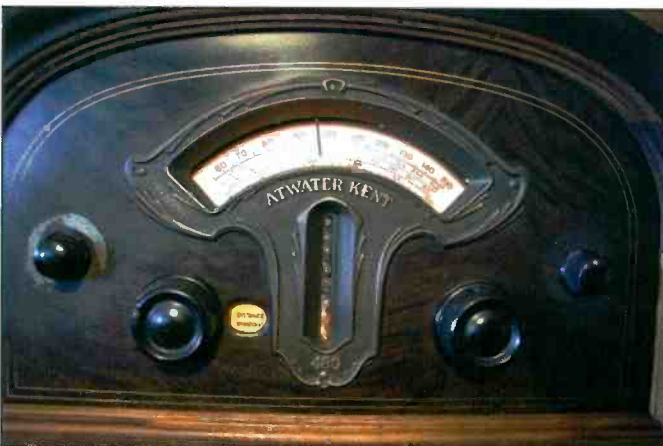
Photo G. A weak signal manages to illuminate three of the neon bulbs.
