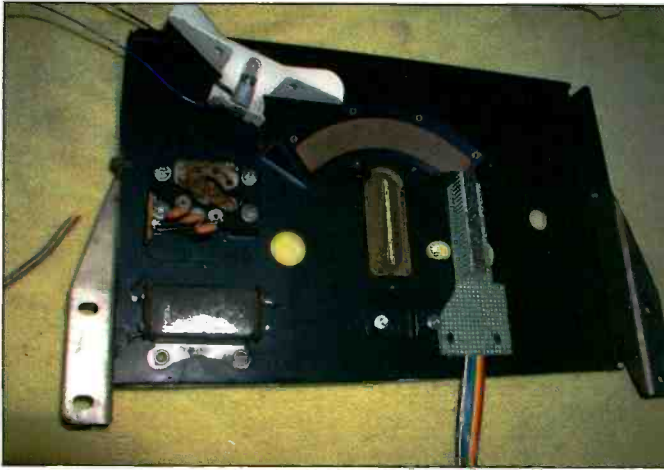
Photo D. The Tonebeam display before it was mounted behind the Tonebeam window in the dial escutcheon.
