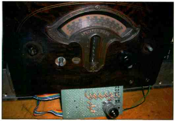
Photo E. The Tonebeam display is installed in the escutcheon and the remainder of the circuit (contained on a small perf board) will be mounted under the chassis.
